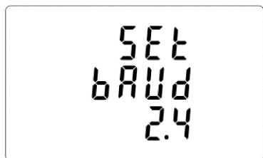
Use **P▼** and **MD/PF/HZ▲** buttons to choose Baud rate: 0.3 / 0.6 / 1.2 / 2.4 / 4.8 / 9.6 [kbps].
