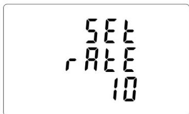
From the setup menu, use and buttons to select the pulse rate option.
