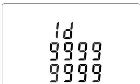
From the setup menu, use **P** and **MD/PF/HZ** buttons to select extended address option.
