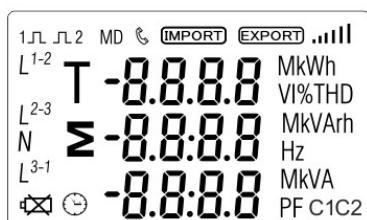
The first screen lights up all display segments and can be used as a display check.
