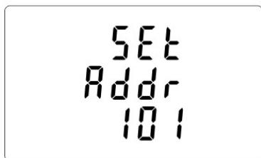
Use **P** and **MD/PF/HZ** to change digits and **E** to change position, to choose Modbus address (001 to 250).
