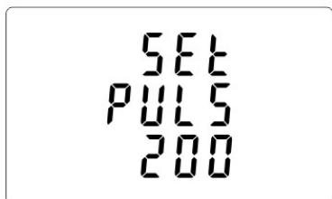
From the setup menu, use and buttons to select the pulse width option.
