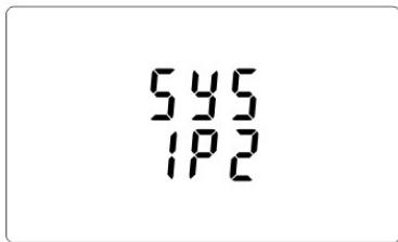
Use **P** and **MD/PF/HZ** buttons to select the required system option: 1P2W, 3P3W, 3P4W.
