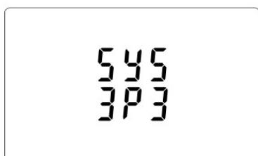
From the set up menu, use **P** and **MD/PF/HZ** buttons to select the system option.
