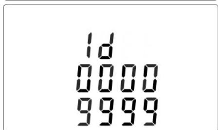
Use **P** and **MD/PF/HZ** buttons to change digits and **E** to change position, to choose Modbus address (00000000 to 99999999).
