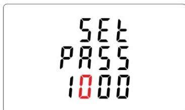
Use **P** and **MD/PF/HZ** buttons to set the first digit and press **E** to confirm your selection. The next digit will flash.
